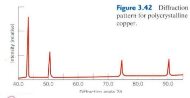
x-ray diffraction pattern for copper, which has an FCC crystal structure; monochromatic x-radiation having a wavelength of 0.1542 nm was used.
